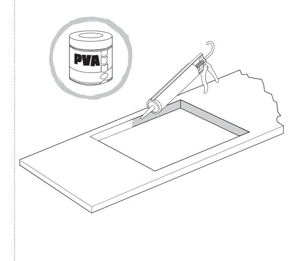
Seal the cut edge of the worktop using silicone sealant or PVA adhesive.
