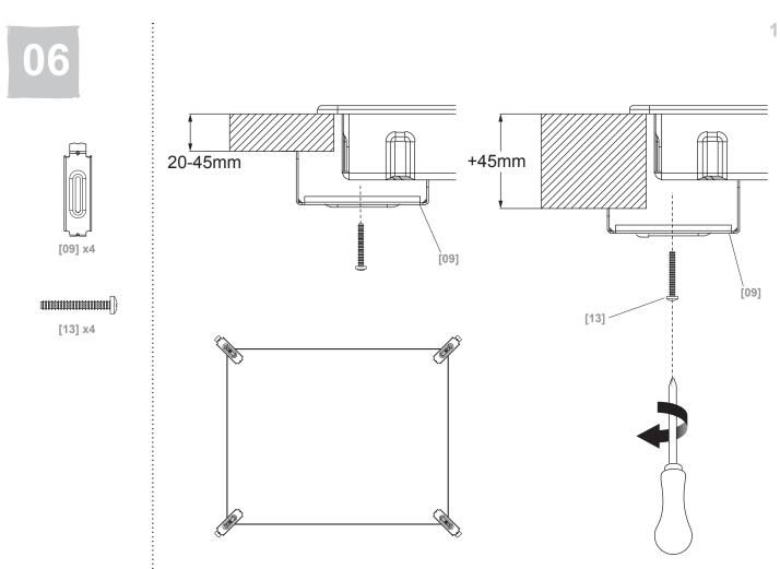
Secure the hob to the worktop by attaching the brackets as shown.
