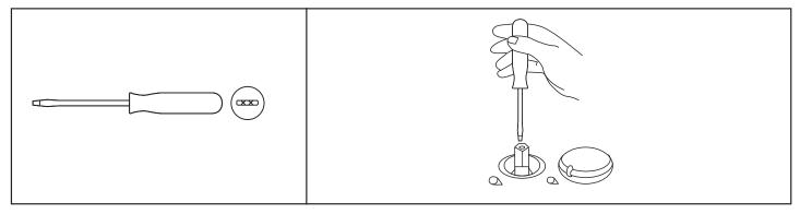
Regulation of the "MINIMUM" position on the burners.
