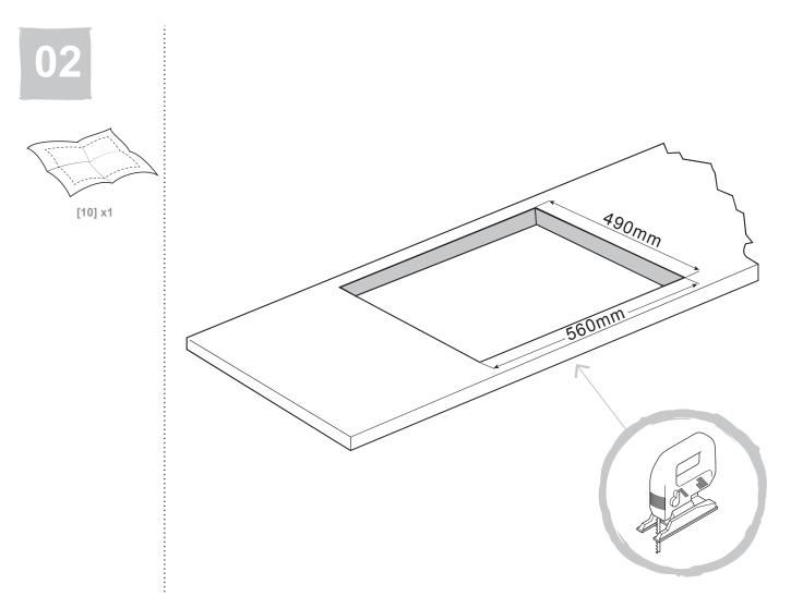
Cut an aperture in the worktop using a jigsaw as shown. The worktop should be at least 30mm thick and made of a heat resistant material.
