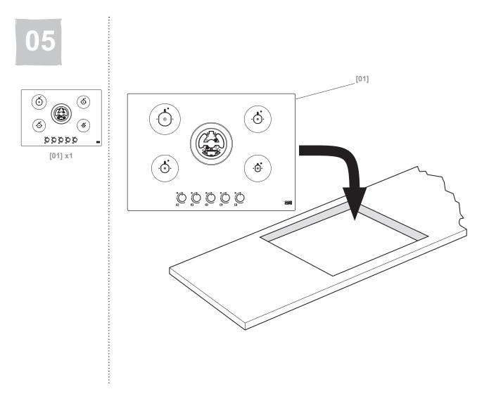
Once the worktop edge has cured, and the tape is fitted, position the hob into the cutout in the worktop.
