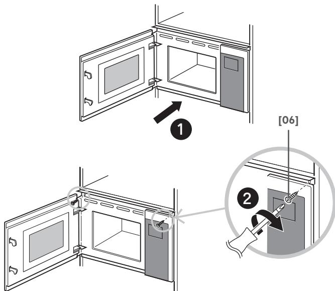
**EN** Carefully slide the microwave into the cabinet ensuring the power cable is not trapped. Secure the top panel to the cabinet using the two screws [06] provided.
