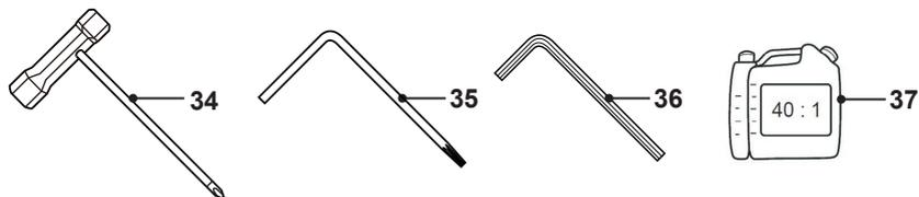
34. Multi-tool I (Cross-head screwdriver/ socket wrench)
