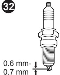
6. Check the spark plug gap. It should be 0.6-0.7 mm (Fig. 32).
